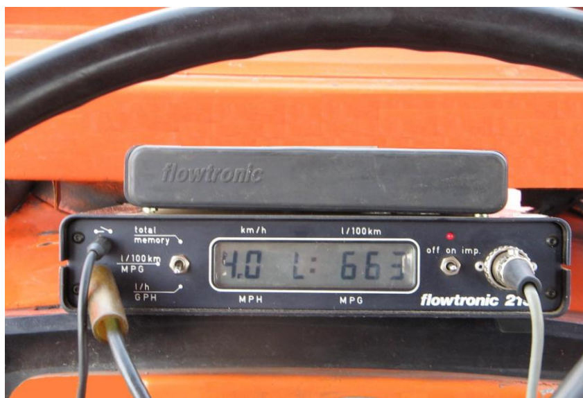
Fig. 1. The device FLOWTRONIC 217 for determining fuel consumption placed on the tractor U-650M
